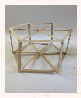
Create the base of the ferris wheel by gluing 7 popsicle sticks together in an eight shape and 4 sticks together with a small x shape on the top
